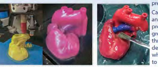
3D printing in progress on desktop Printrbot (left) and Connex3 (right). Applying resin to protect ColorJet print.
